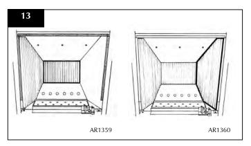
• Locate the top panel on top of the sides and rear by lifting it up and forward inside the box.
